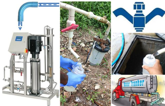
RO purifiers are high pressure semipermeable membrane systems. Basic schema of a RO system consists of pre- and post-treatment units around the core RO unit. Pre-treated water is fed into RO unit under high pressure. Water that permeates through the RO membrane comes out as the product water, and the remaining concentrated water comes out as the reject water. The quality of feed water affects RO system performance and cost of
